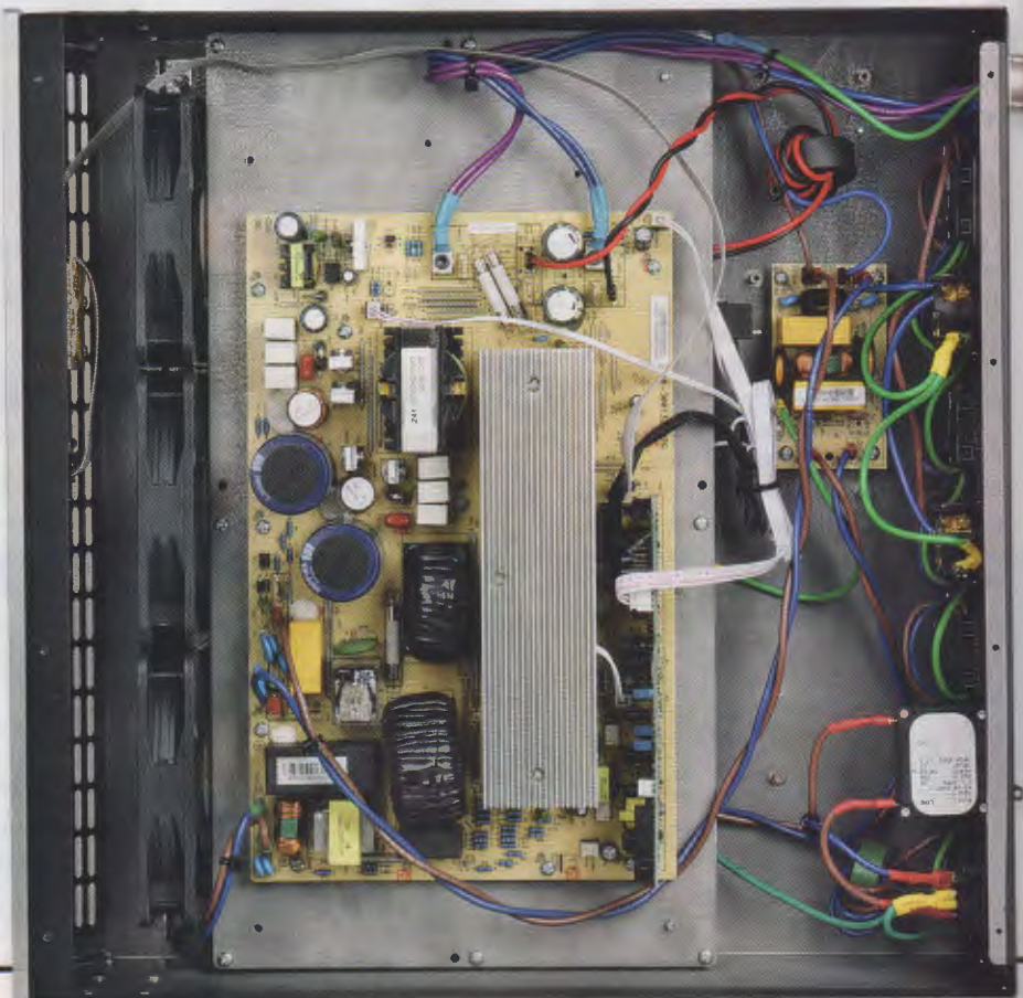
RIGHT: Compared to the PS Audio P10, there is plenty of empty space within the 2000HV's Regenerator box, and its amplifier makes do with a surprisingly small heatsink
